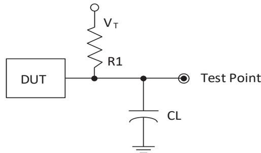
**Figure 3.9. Output Test Load, LVTTTL and LVCMOS Standards**
