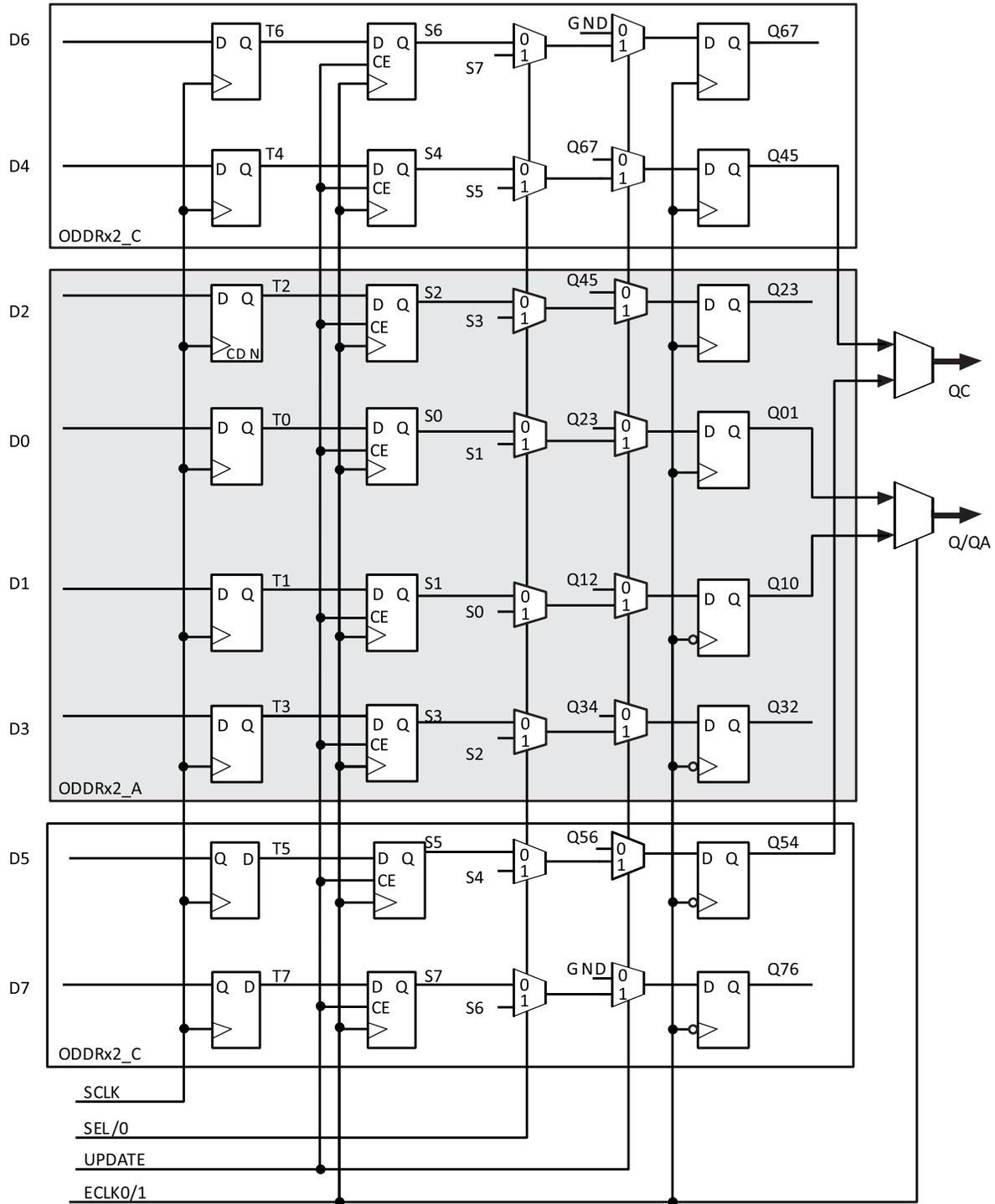
Figure 2.13. Output Gearbox
