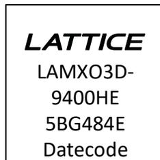
**Figure 5.2. Top Markings for Automotive Grade Devices**
