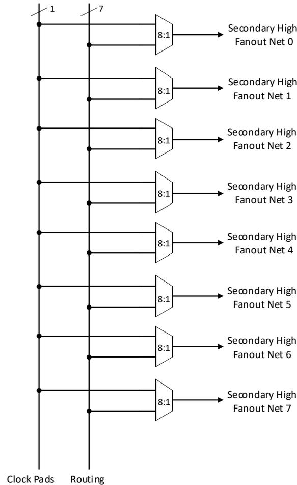
**Figure 2.5. Secondary High Fanout Nets for MachXO3D Devices**
