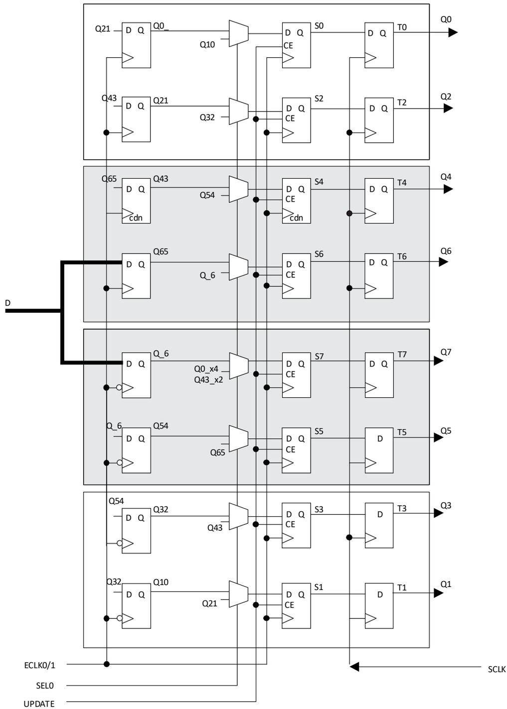
Figure 2.12. Input Gearbox
