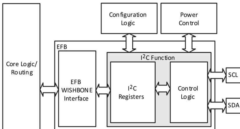
Figure 2.17. I<sup>2</sup>C Core Block Diagram
