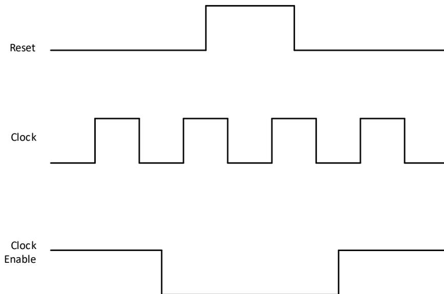
**Figure 2.9. EBR Asynchronous Reset (Including GSR) Timing Diagram**
