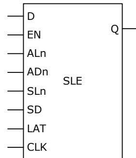
The following figure shows a configuration with SD = 0 (synchronous clear) and ADn = 1 (asynchronous clear) for a flip-flop (LAT = 0).
