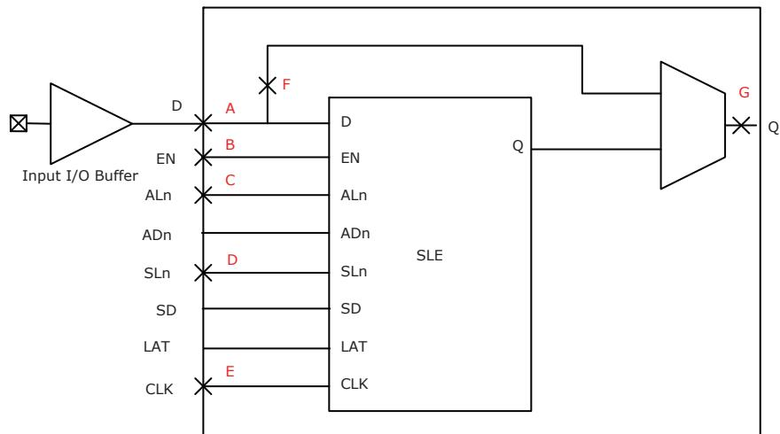
**FIGURE 3-7: I/O REGISTER INPUT TIMING DIAGRAM**
