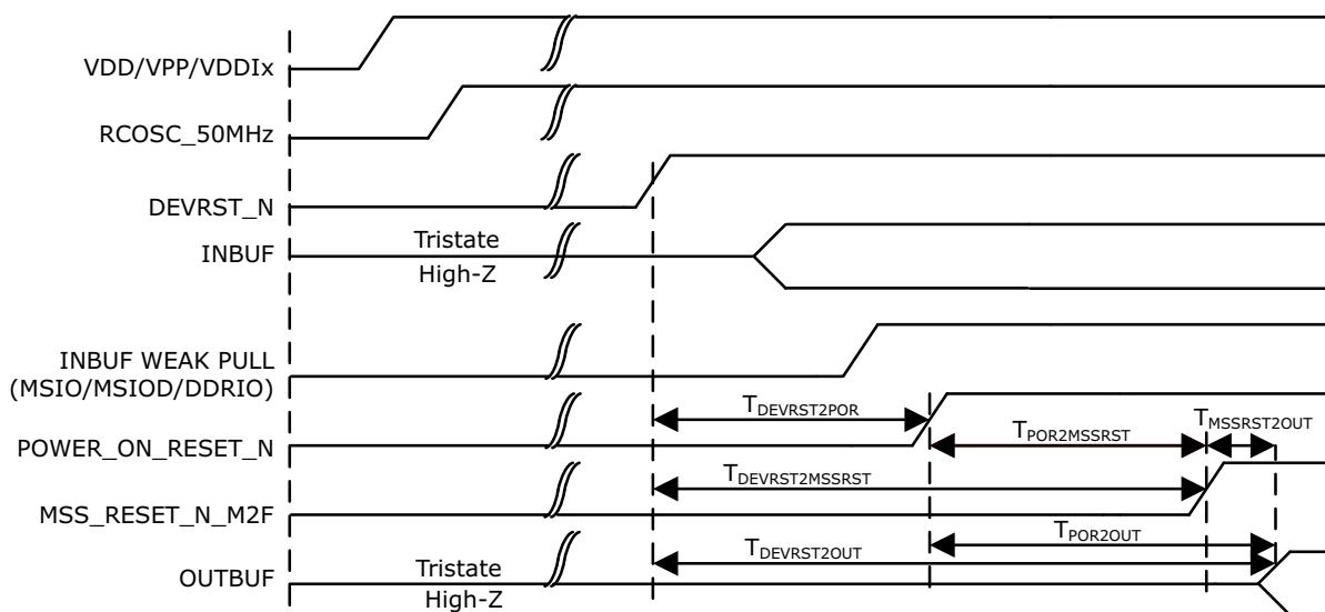
**FIGURE 3-20: DEVRST\_N TO FUNCTIONAL TIMING DIAGRAM FOR IGLOO 2**
